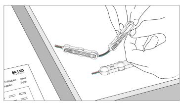
2 Remove the tape from the back of the LEDs and stick them in place according to the provided LED layout, including the appropriate module pitch (refer to Figure 1 on page 2).
