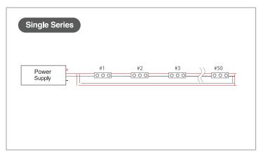
Do not exceed the maximum number of LED modules per series (refer to each item's spec sheet for specific numbers). We recommend wiring both ends of LED modules to the power supply.
