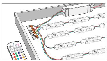
Wire both ends of LED modules to the controller and power supply. For multiple series, connect them in parallel to avoid voltage drop (refer to page 2).
